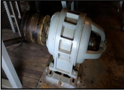
This photo is of a raw hide pulley installed on one of the electric motors.
